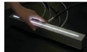
335mm linear plasma source for surface treatment
